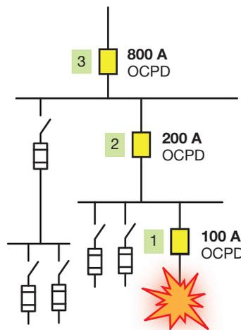
**Figure 2** In a selectively coordinated system, only the 100 A-rated device at location 1 would open to clear this branch circuit fault.
